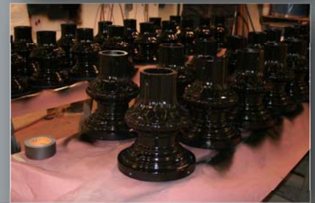
Light Pole Bases Sandblast SSPC-10 Epoxy Primer Urethane Finish
